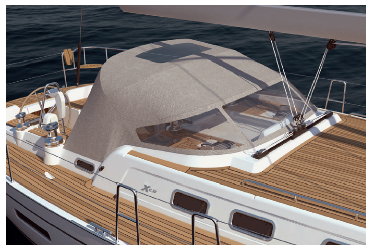
The standard spray hood is supported by stainless steel frames. Standard colour is Taupe (Swela 37329). For canvas colour options, see page 17.
