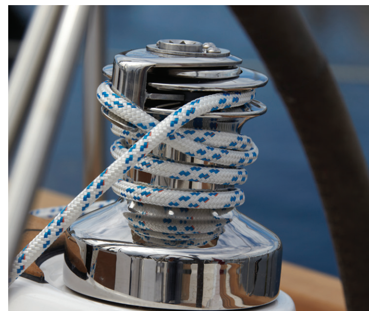
Stainless steel self-tailing Andersen Winches, which can be upgraded to be electrical powered are part of Xc 38's comprehensive standard quality.
