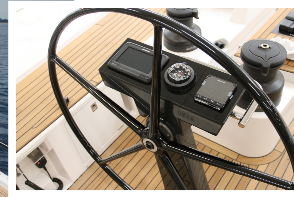
Small instrument mount with grab-rail
