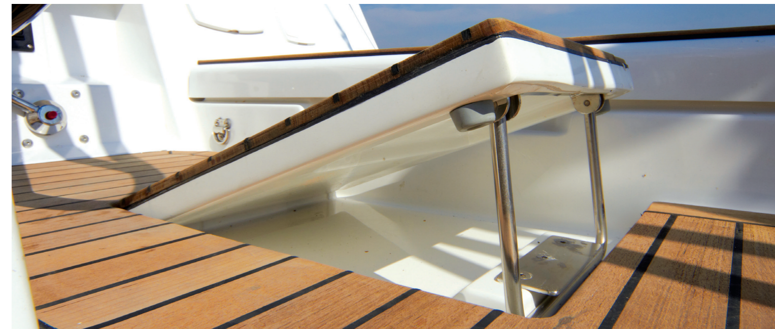
Adjustable folding foot chocks
