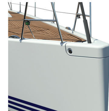
Optional GRP cowl for rating efficiency
